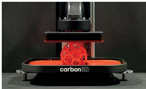
Carbon3D technology uses light and oxygen to grow objects from a pool of resin
