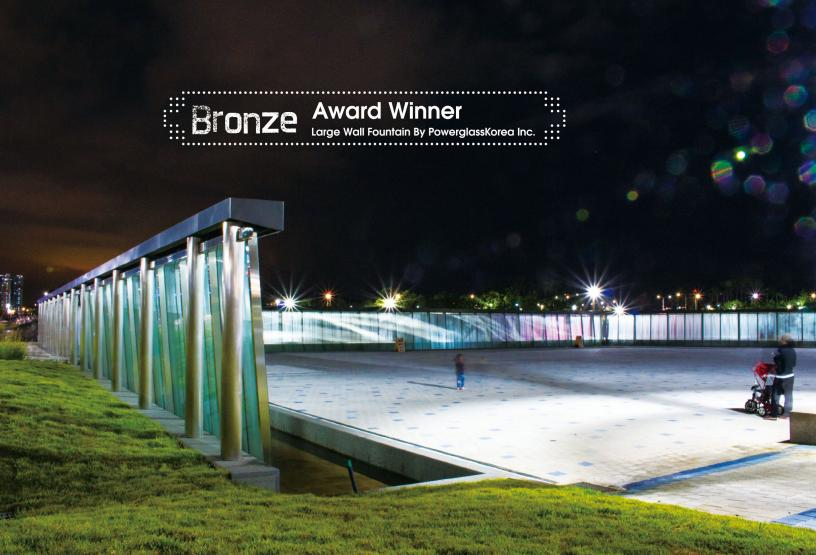
They say people can't walk on water, but the team at powerglasskorea have proved beyond a doubt that you can draw on it. Using a special watertight conductor to avoid exposing the wires, LED images are displayed on a transparent glass wall, creating the illusion that figures are being actually displayed on water. The sheer length of this wall – more than 100m in total – also makes this feature all the more impressive.
